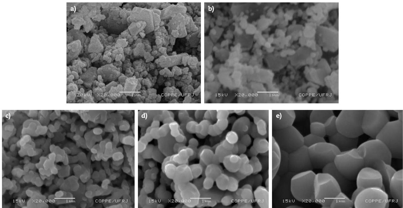
**Fig. 1 – (a) Microstructure of the green body; (b) no significant changes were observed at 1,000 °C; (c), (d) and (e) the pellets consisted of a fine particle network surrounded by big voids with extensive necking between particles, whose size increases with temperature, respectively at 1,200 °C, 1,400 °C and 1,600 °C.**
