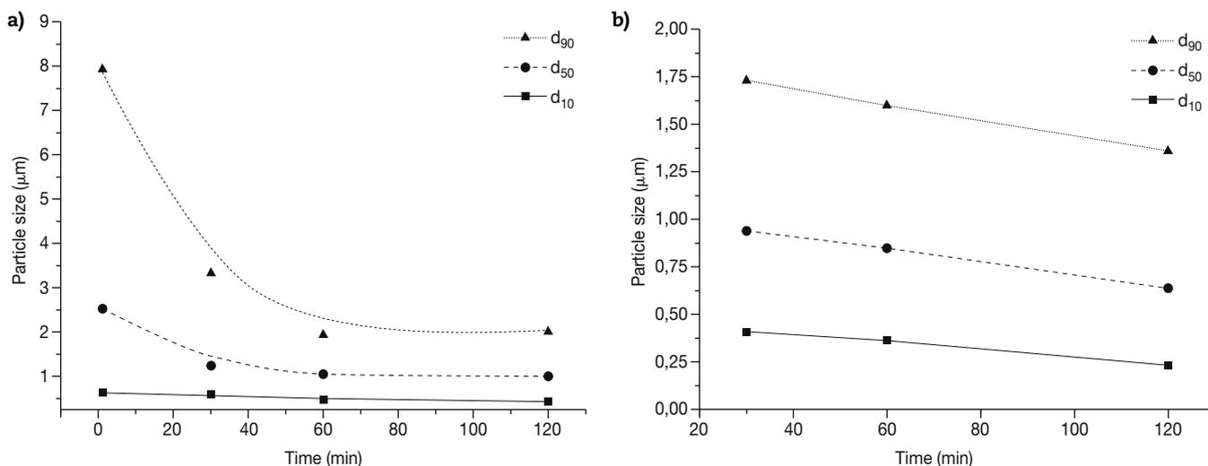
**Fig. 4 – d<sub>10</sub>, d<sub>50</sub> and d<sub>90</sub> particle size distribution of (a) Al<sub>2</sub>O<sub>3</sub> and Y<sub>2</sub>O<sub>3</sub> and (b) Al<sub>2</sub>O<sub>3</sub> and yttrium aluminum garnet powders with milling time.**
