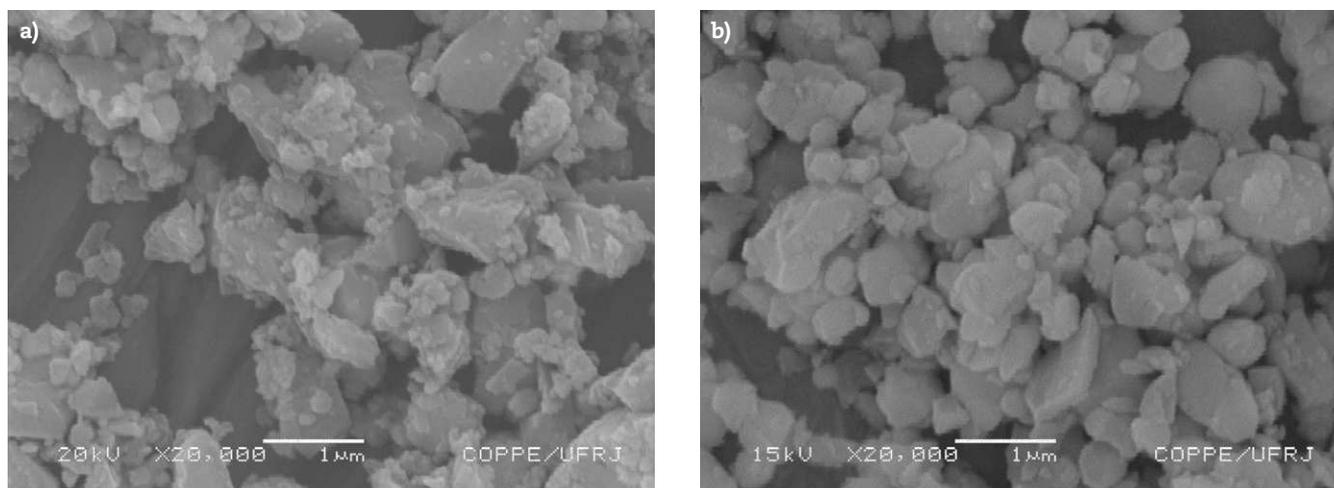
**Fig. 5 – Scanning electron microscope secondary electron, 20,000× magnification of (a)  $\text{Al}_2\text{O}_3\text{-Y}_2\text{O}_3$  mixture milled for 120 min; (b)  $\text{Al}_2\text{O}_3\text{-yttrium aluminum garnet}$  mixture milled for 120 min.**
