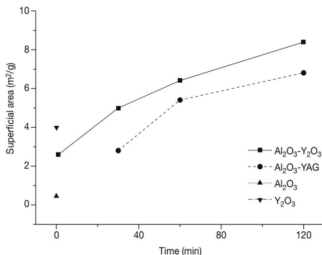
**Fig. 3 – BET superficial area variation with milling time of the Al<sub>2</sub>O<sub>3</sub>-Y<sub>2</sub>O<sub>3</sub> mixture.**
