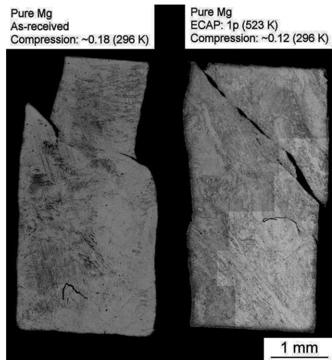
**Fig. 5 – Grain structure along the longitudinal section of the workpieces of the (left) as-received material and (right) material processed by ECAP after being tested in compression at room temperature up to failure.**
