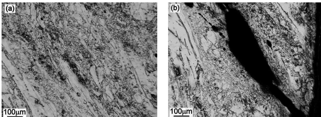
**Fig. 6 – Grain structure of pure magnesium processed by ECAP and subjected to compression along the axial direction (vertical direction in the images). Alternating bands of refined grains and coarse grains (a) away from the fracture and (b) fracture along bands of refined grains.**
