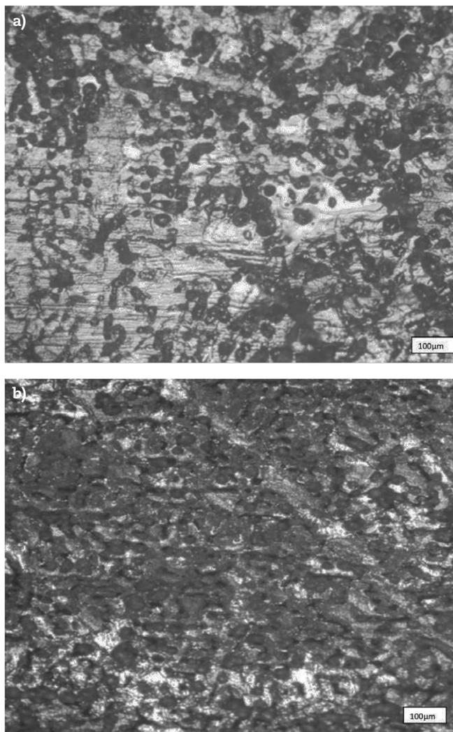
**Fig. 1** – a) Photomicrograph of the Al-Mg-Si/10 wt%  $\text{Al}_2\text{O}_3$  composite showing the  $\text{Al}_2\text{O}_3$  particles dispersed in the Al-Mg-Si matrix. b) Photomicrograph of the Al-Mg-Si/4wt% rice husk ash-6 wt%  $\text{Al}_2\text{O}_3$  hybrid composite showing a high density of particles dispersed in the Al-Mg-Si matrix.
