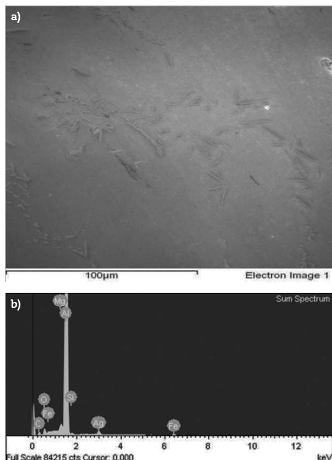
**Fig. 2** – a) Representative SEM photomicrograph of the Al-Mg-Si/2wt% rice husk ash-8 wt%  $\text{Al}_2\text{O}_3$  hybrid composite showing particles dispersed in the Al-Mg-Si matrix. b) EDAX profile obtained from the Al-Mg-Si/2wt% rice husk ash-8 wt%  $\text{Al}_2\text{O}_3$  hybrid composite confirming the presence of  $\text{Al}_2\text{O}_3$ ,  $\text{SiO}_2$ ,  $\text{Fe}_2\text{O}_3$ ,  $\text{K}_2\text{O}$ , C, and Ag.
