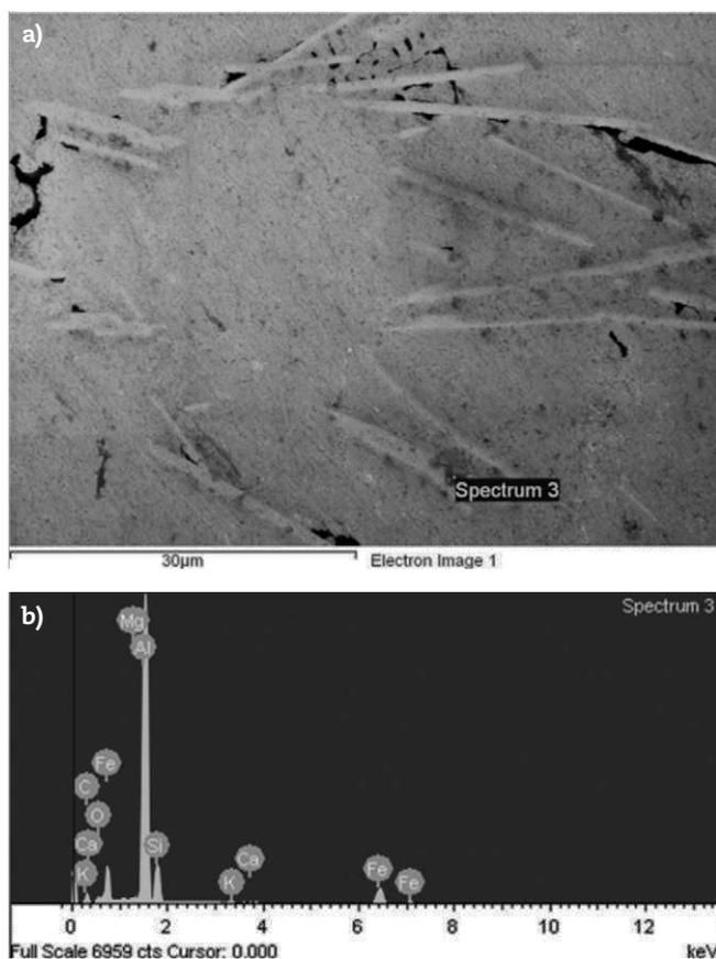
**Fig. 3 – a) Representative scanning electron microscope photomicrograph of the Al-Mg-Si/3wt% rice husk ash-7 wt% Al<sub>2</sub>O<sub>3</sub> hybrid composite showing particles dispersed in the Al-Mg-Si matrix. b) EDAX profile obtained from the particle identified in (a) confirming the presence of Al<sub>2</sub>O<sub>3</sub>, SiO<sub>2</sub>, Fe<sub>2</sub>O<sub>3</sub>, K<sub>2</sub>O, Cao, and C which are known constituents of rice husk ash.**
