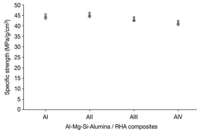
**Fig. 6 – Variation of specific strength for the single reinforced Al-Mg-Si/10 wt%  $\text{Al}_2\text{O}_3$  and hybrid reinforced Al-Mg-Si/rice husk ash- $\text{Al}_2\text{O}_3$  composites. RHA: rice husk ash.**
