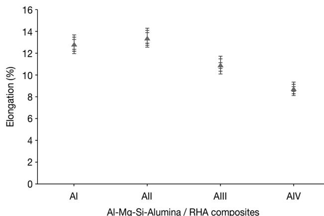
**Fig. 7 – Variation of percent elongation for the single reinforced Al-Mg-Si/10 wt%  $\text{Al}_2\text{O}_3$  and hybrid reinforced Al-Mg-Si/rice husk ash- $\text{Al}_2\text{O}_3$  composites. RHA: rice husk ash.**
