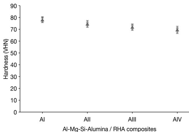
**Fig. 4 – Variation of hardness for the single reinforced Al-Mg-Si/10 wt% Al<sub>2</sub>O<sub>3</sub> and hybrid reinforced Al-Mg-Si/rice husk ash-Al<sub>2</sub>O<sub>3</sub> composites.**
