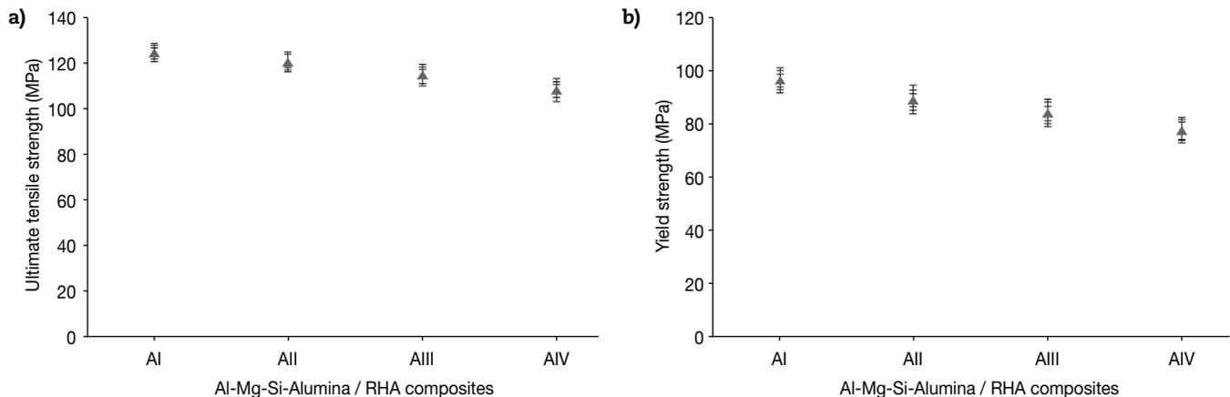
**Fig. 5 – a) Variation of tensile strength for the single reinforced Al-Mg-Si/10 wt%  $\text{Al}_2\text{O}_3$  and hybrid reinforced Al-Mg-Si/rice husk ash- $\text{Al}_2\text{O}_3$  composites. b) Variation of yield strength for the single reinforced Al-Mg-Si/10 wt%  $\text{Al}_2\text{O}_3$  and hybrid reinforced Al-Mg-Si/rice husk ash- $\text{Al}_2\text{O}_3$  composites.**
