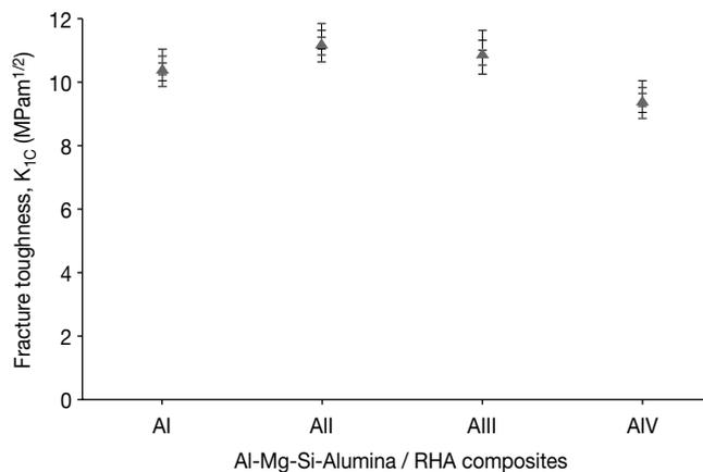
**Fig. 8 – Variation of fracture toughness for the single reinforced Al-Mg-Si/10 wt%  $\text{Al}_2\text{O}_3$  and hybrid reinforced Al-Mg-Si/rice husk ash- $\text{Al}_2\text{O}_3$  composites. RHA: rice husk ash.**
