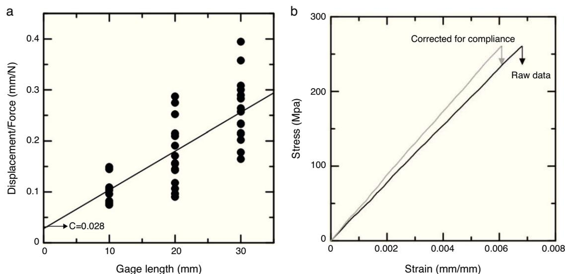
**Fig. 5 – Determination of the machine compliance: (a) displacement/force versus gage length. The machine compliance, given by the intercept ( $c=0.028$ ), was determined from this plot, (b) stress-strain behavior of a jute fiber tested at a 40 mm gage length, showing the “as measured” data and that corrected for compliance.**
