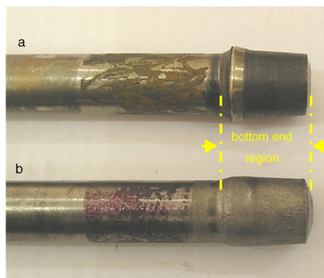
Fig. 5 – The bottom end region of (a) an unused (wear-free) and (b) a wearing rod part.
