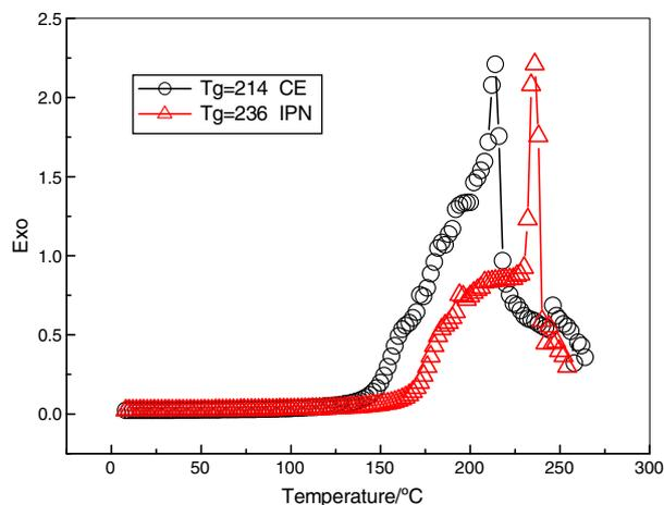
**Fig. 4 – DSC curves of the vitrification temperature.**
