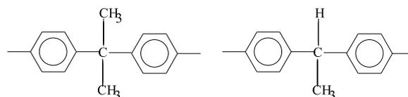
CE was in situ polymerized (curing) into polycyanurate (PCN) at high temperature under the action of catalyst. PCN has many advantages of good toughness, higher glass transition temperature ( $T_g$ ), lower dielectric constant and loss factor, lower water absorption rate, and inherent flame retardancy. At high temperature (220–270 °C), its molten body is chemically
