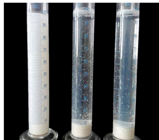
Fig. 5 – Effect of chitosan on the settling behavior of quartz at different pH (settling time = 5 min; left: pH = 3, middle and right: pH = 9).
