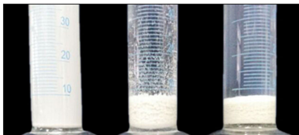
Fig. 6 – Effect of the change of pH on the settling behavior of quartz (settling time = 60 min; left: pH 3, middle: pH 9, right: pH 9-3).
