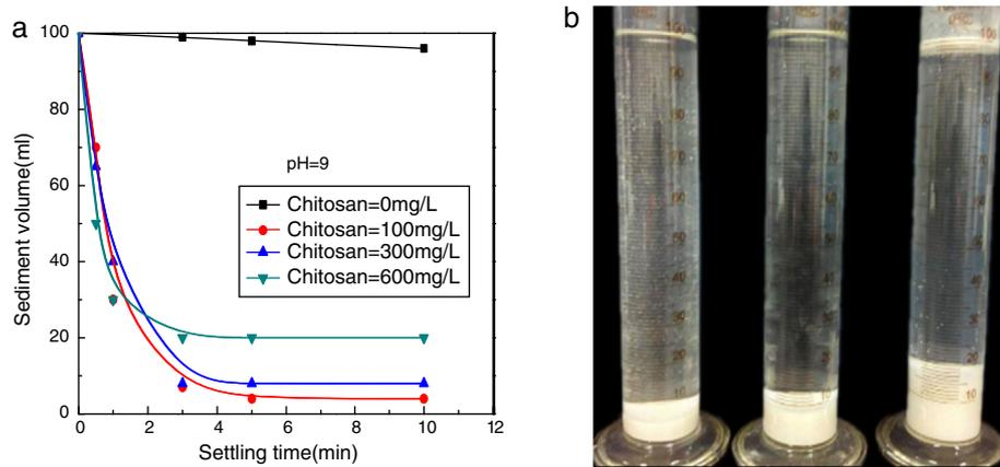
**Fig. 4 – (a) Effect of chitosan amount on the settling behavior of quartz at pH 9. (b) Photograph at the settling time of 3 min. The dosage of chitosan from left to right is 100 mg/L, 300 mg/L, 600 mg/L.**
