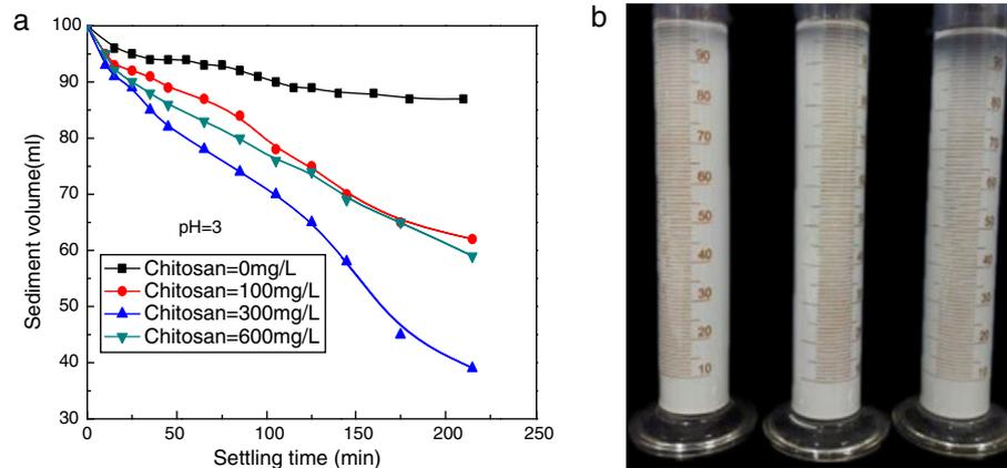
**Fig. 3 – (a) Effect of chitosan amount on the settling behavior of quartz at pH 3. (b) Photograph at the settling time of 30 min. The dosage of chitosan from left to right is 100 mg/L, 300 mg/L, 600 mg/L, respectively.**
