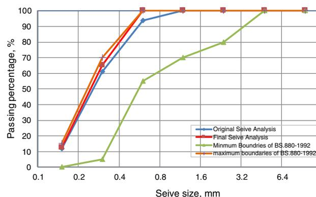
**Figure 1 – Grading curve of the sand.**
