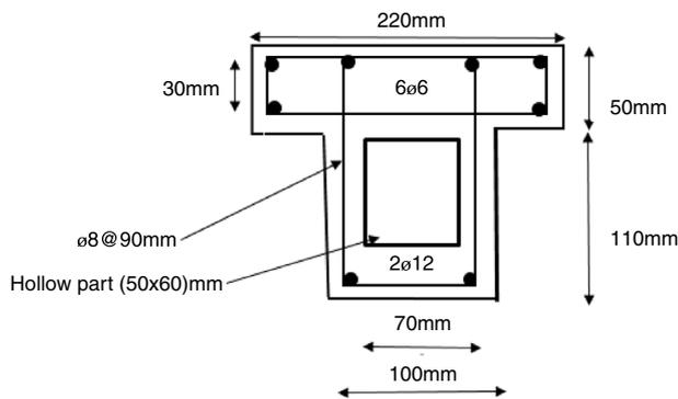
Figure 5 – Section B-B; showing rebar's details.
