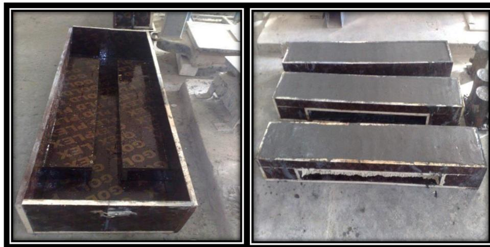
Figure 6 - Plywood molds.
