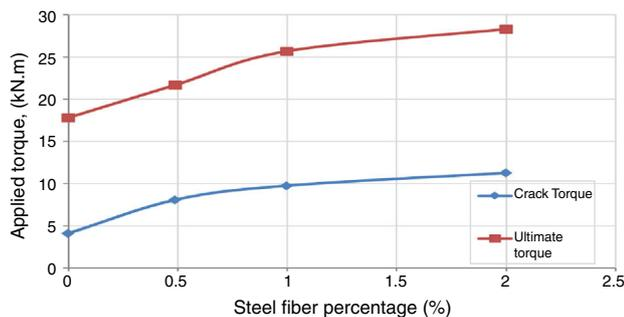
**Figure 8 – Crack ( $T_{cr}$ ) and ultimate ( $T_{ult}$ ) torques of RPC hollow T-beams.**
