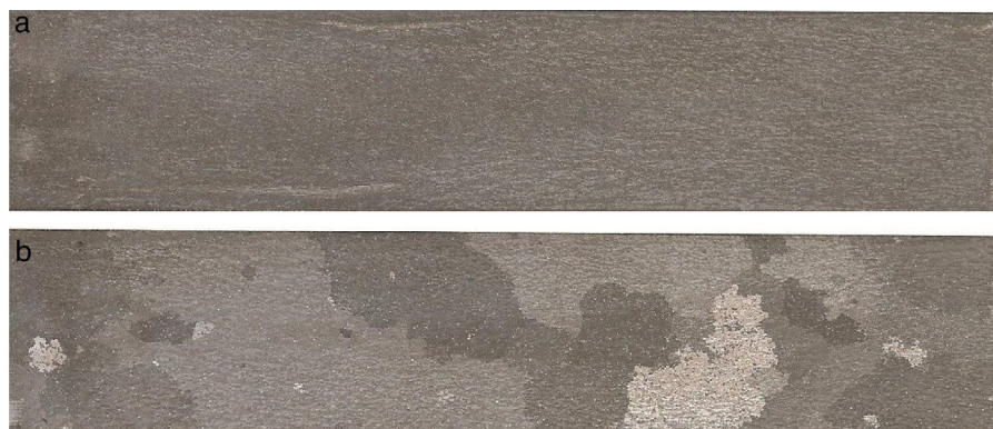
Fig. 4 – Macrostructure of samples annealed at (a) 1070 °C and (b) 1080 °C with interruption.
