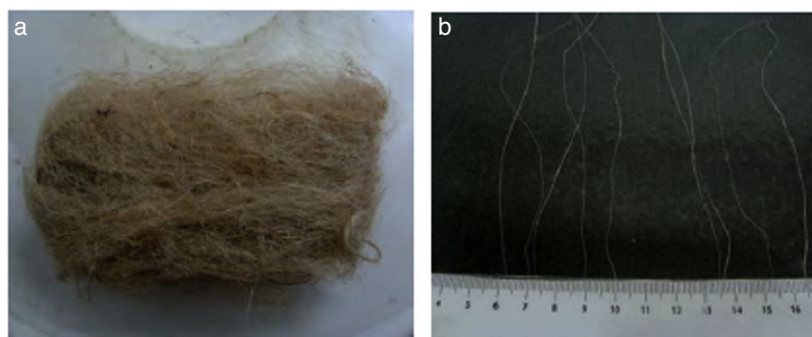
Fig. 1 – A bundle of as-received (a) and individually separated jute fibers (b).
