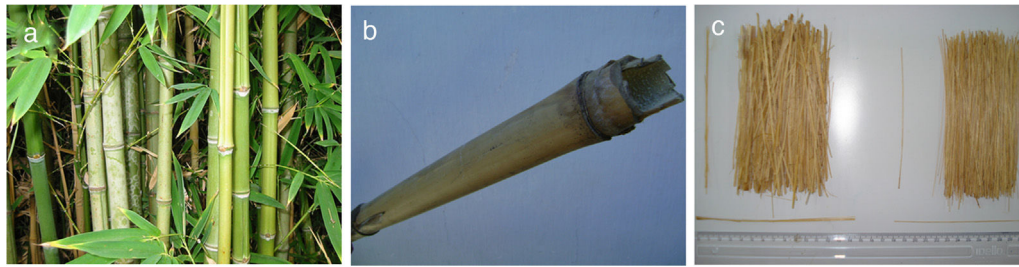
Fig. 1 – Bamboo trees (a), dried bamboo culm (b) and its fibers longitudinally stripped with different diameters (c).
