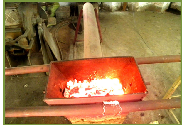
Fig. 3 – Top burning bed of sinter of laboratory grade sintering machine.
