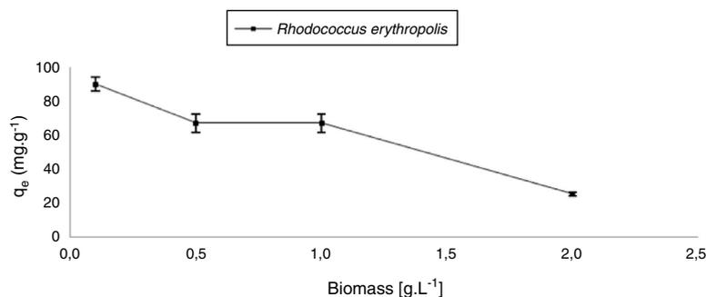
**Fig. 3 – Effect of biomass concentration on copper biosorption ([Cu<sup>2+</sup>] = 100 mg L<sup>-1</sup>, pH 6, t<sub>contact</sub> = 120 min).**
