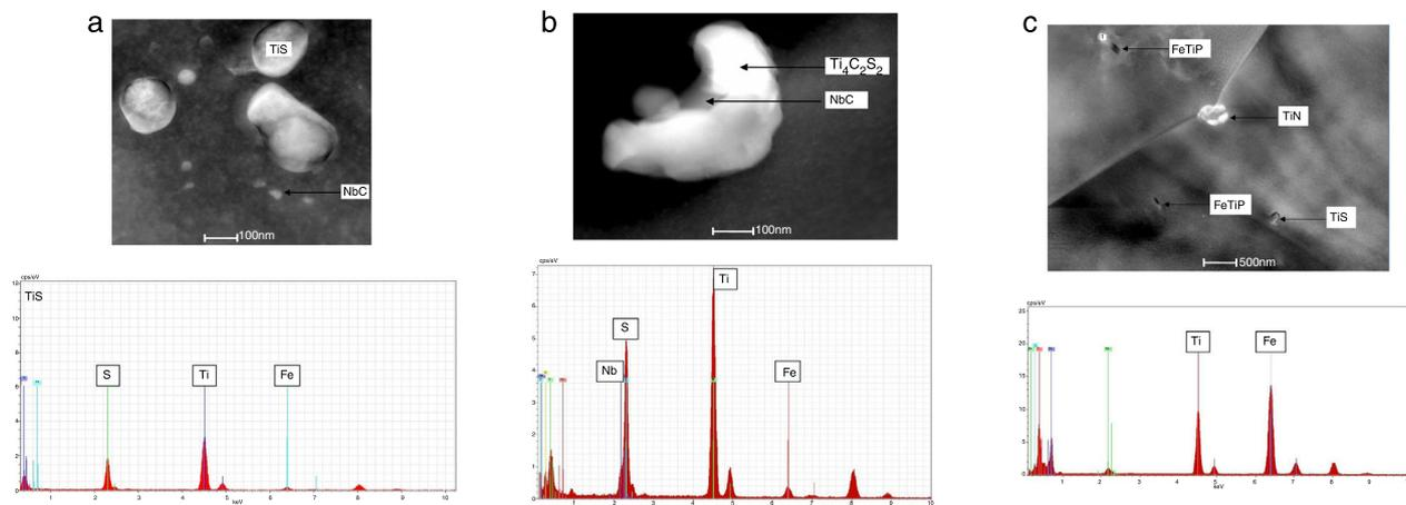
**Fig. 3 – The main precipitates found in: (a) IF-Ti, (b) IF-TiNb, (c) IF-TiNbP.**
