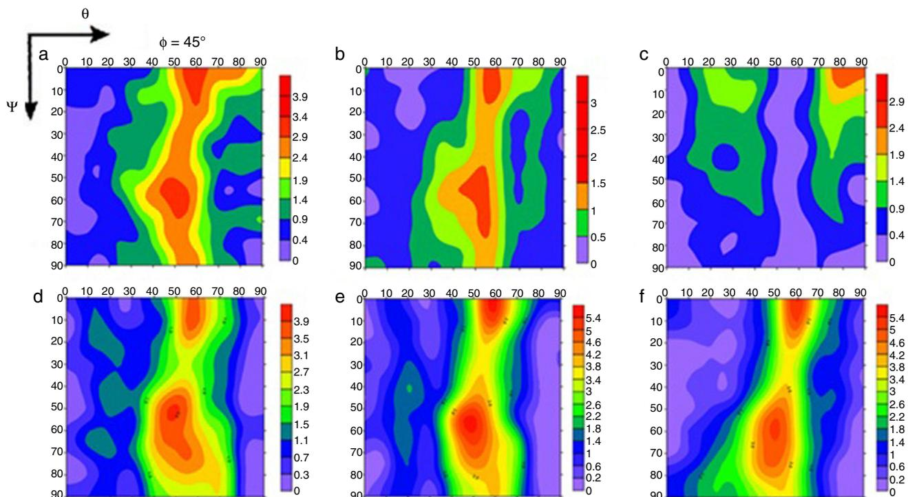
**Fig. 4 – ODF's of the samples: measurements on the surface of (a) IF-Ti steel, (b) IF-TiNb steel, (c) IF-TiNbP steel; measurements in the half thickness, (d) IF-TiNb steel, (e) IF-TiNbP steel, (f) IF-TiNbP steel.**
